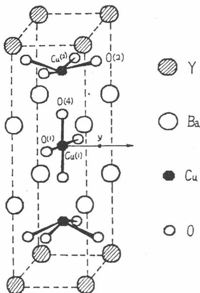
Figure 1. The crystal structure of  $\text{LaBa}_2\text{Cu}_3\text{O}_y$ .
