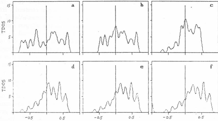
Figure 4. Total densities of states for  $\text{LaBa}_2\text{Cu}_3\text{O}_y$ : (a)  $y = 6.6$ , (b)  $y = 6.7$ , (c)  $y = 6.9$ , (d)  $y = 7.0$ , (e)  $y = 7.3$ , (f)  $y = 7.4$ .
