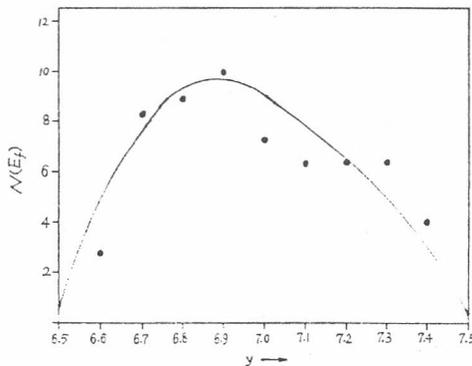
Figure 5. The relationship between  $N(E_f)$  and the  $y$  value in  $\text{LaBa}_2\text{Cu}_3\text{O}_y$ : The circle represents  $N(E_f)$ .
