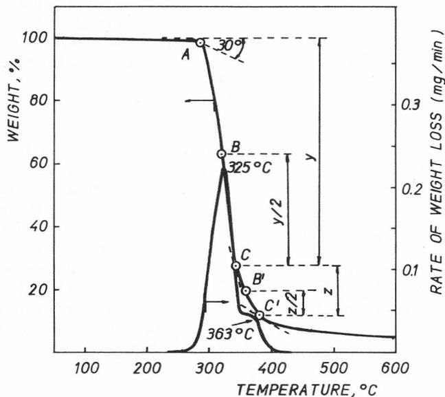
Figure 10. Thermogravimetric analysis of poly(styrene-co-pentabromophenyl methacrylate) (molar ratio 56.5/43.5) in nitrogen.
