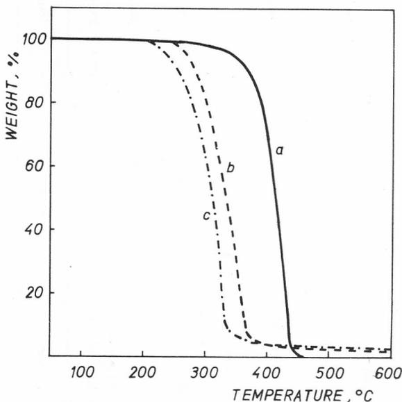
Figure 8. Thermogravimetric analysis of polystyrene (a), poly(2,4,6-tribromophenyl methacrylate) (b), and poly(pentabromophenyl methacrylate) (c) in nitrogen.
