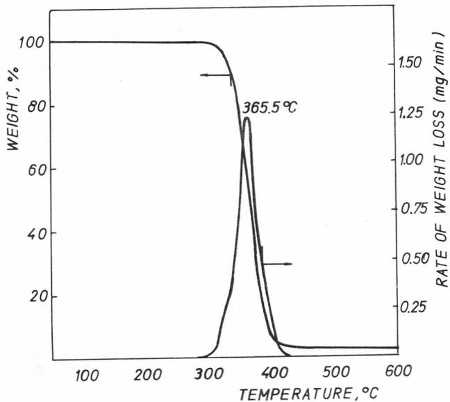
Figure 9. Thermogravimetric analysis of poly(styrene-co-2,4,6-tribromophenyl methacrylate) (molar ratio 55/45) in nitrogen.
