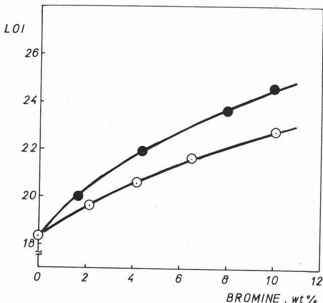
Figure 11. The influence of the content of the brominated monomer (Br wt%) on the limiting oxygen index of poly(styrene-co-2,4,6-tribromophenyl methacrylate) (○) and poly(styrene-co-pentabromophenyl methacrylate) (●).
