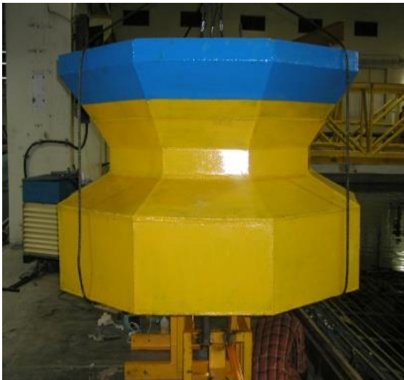
Fig.3 Model without damping plate
