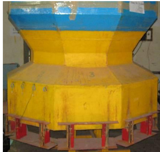
Fig.4 FPSO model with damping plates
