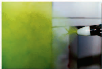
SLIKA 9. Elektrostatičko nabijanje praška – corona-proces 13, 14 FIGURE 9. Electrostatic charging of powder – corona procedure 13, 14
