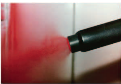
SLIKA 10. Tribo-sustav nabijanja praška 13, 14 FIGURE 10. The tribo-system of powder charging 13, 14
