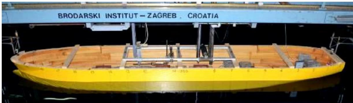
Fig. 2 Towing tank experiment with tanker model [20]
