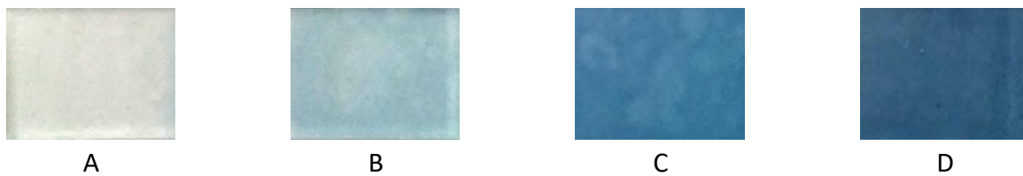
Figure 4. Photographs of ECD A: bleached at +2.5 V, B: colored at -1.5 V, C: -2 V and D: -2.5 V.
