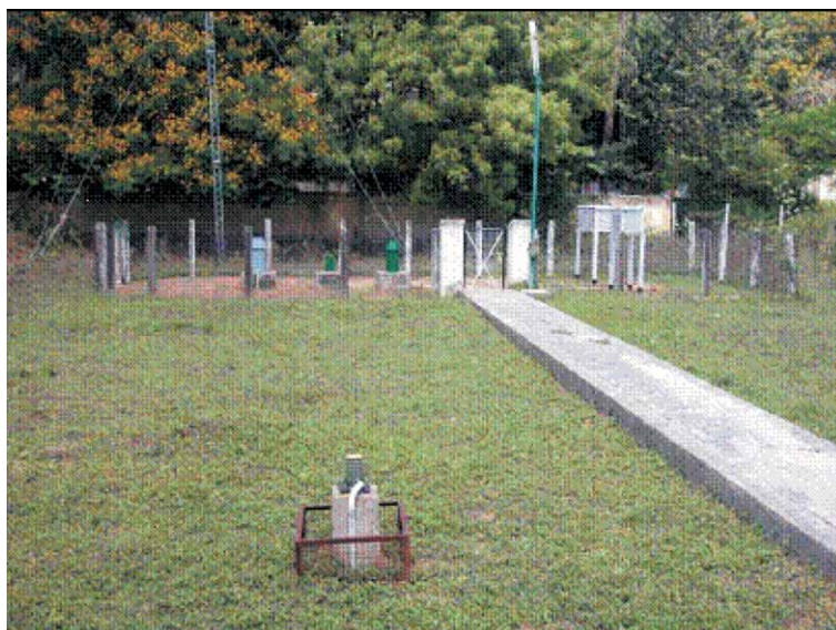
Figure 1. Picture of the disdrometer site, showing relative positions of the JWD and the rain gauge. The JWD is installed in the foreground while the rain gauge may be observed in the background in blue inside the fenced in observation area. The JWD is actually about 25 m to the east of the SRRG.
