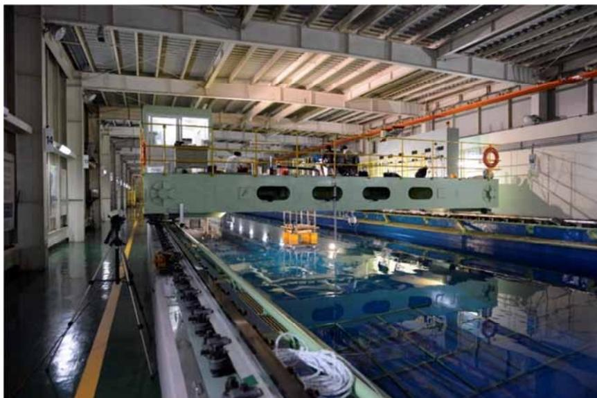
Fig. 2 Photo of the towing carriage with the TLP model
