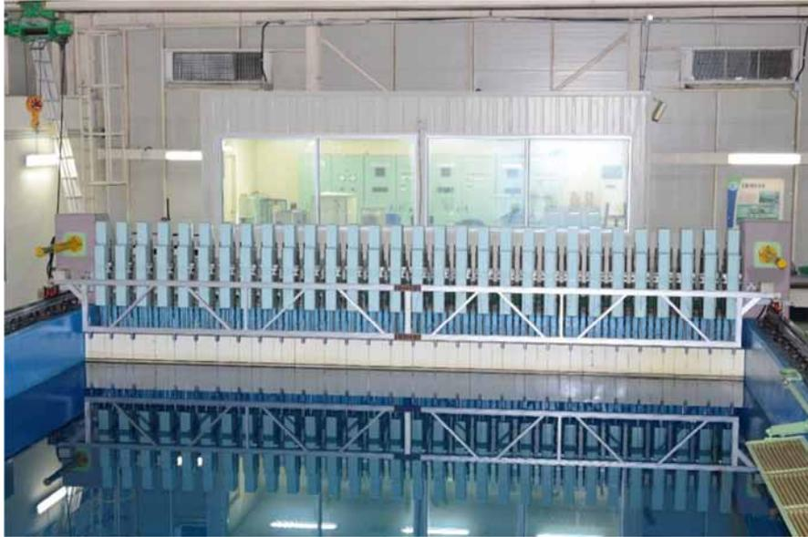
Fig. 3 Photo of the wavemaker and the control room
