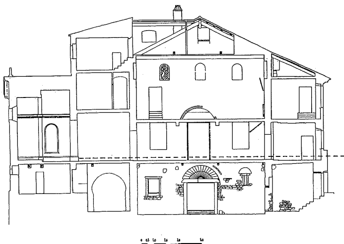
Fig. 5., Poreč, Episcopal Palace, transverse section, view to the south (the original position of the floor is marked)
