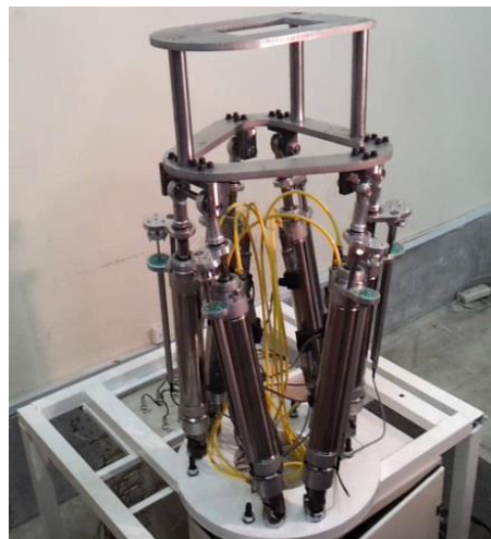
Fig. 1. The University of K. N. Toosi parallel robot for lower limb rehabilitation
