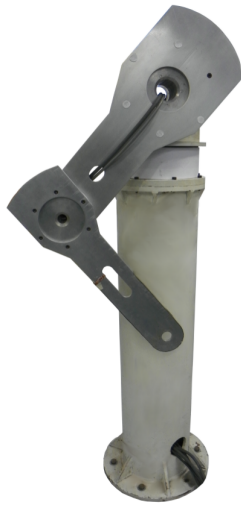
Fig. 3. Experimental robot manipulator “Rotradi”
