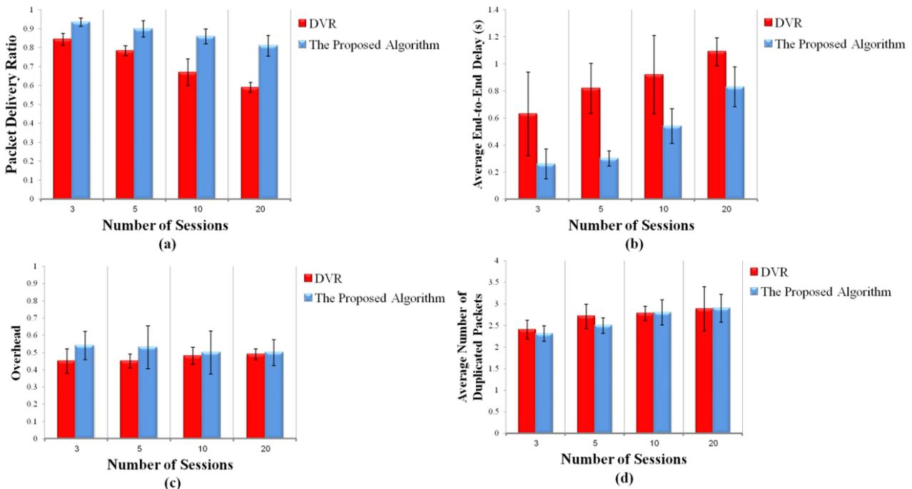
Fig. 6. (a) Data Delivery Ratio, (b) Average End-to-End Delay, (c) Overhead, and (d) Duplicated Packets versus the number of communication sessions
