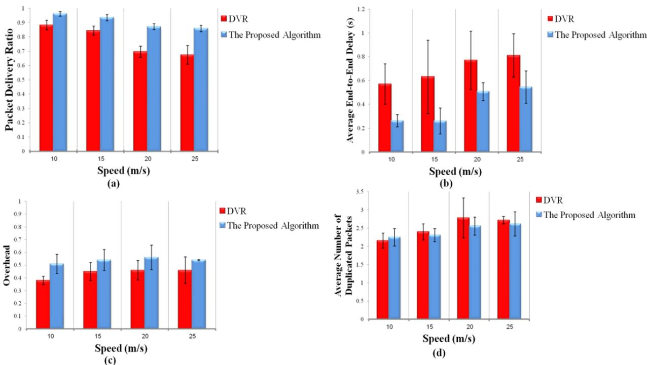
Fig. 4. (a) Data Delivery Ratio, (b) Average End-to-End Delay, (c) Overhead, and (d) Duplicated Packets versus nodes' speed of mobility
