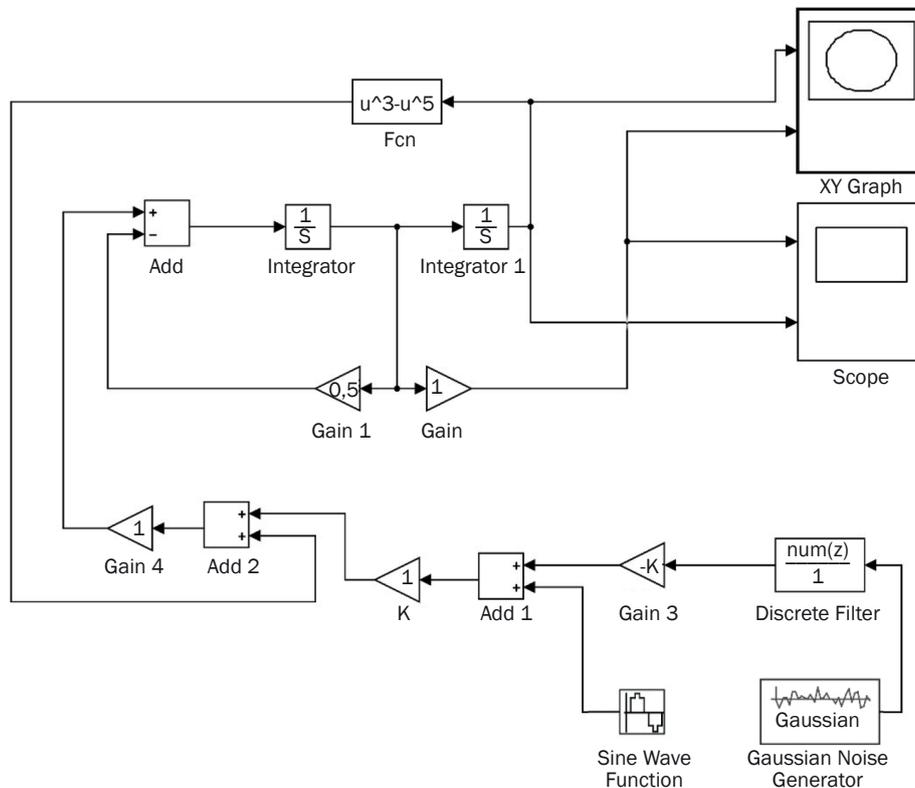
Figure 1 - MATLAB model of Duffing's dynamic system
