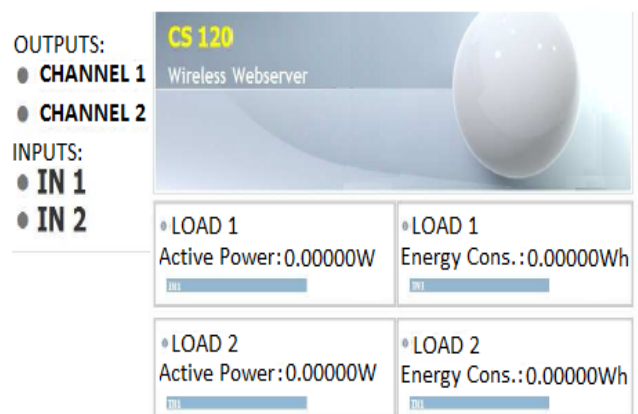
Fig. 18. Screenshot of realized web page in order to switch on/off the connected electrical loads and view, after current data processing, instantaneous active power (W) and overall consumed energy (Wh).
