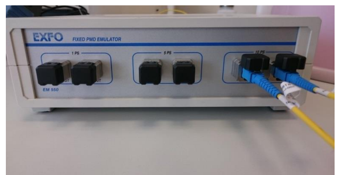
Fig. 10. PMD emulator including 1, 5 and 10 ps delay lines.
