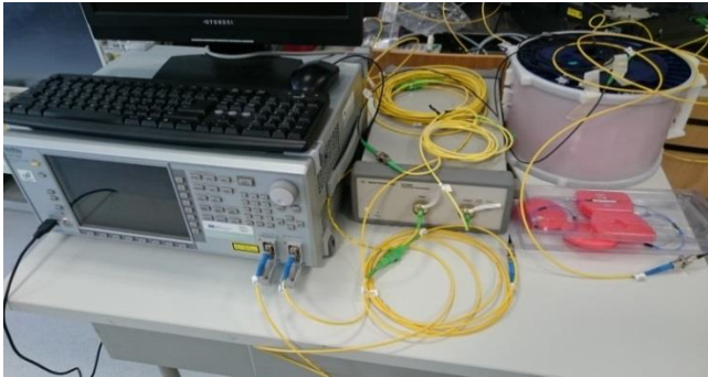
Fig. 7. The measurement workplace for the Fixed Analyzer method.
