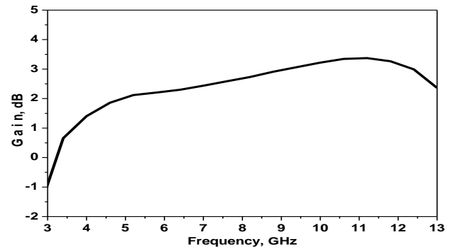
Fig. 11. Gain in dB of our antenna against frequency
