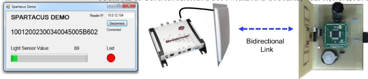
Fig. 9. The SPARTACUS demo running on a general-purpose PC connected to the Impinj Speedway Revolution RFID reader.
