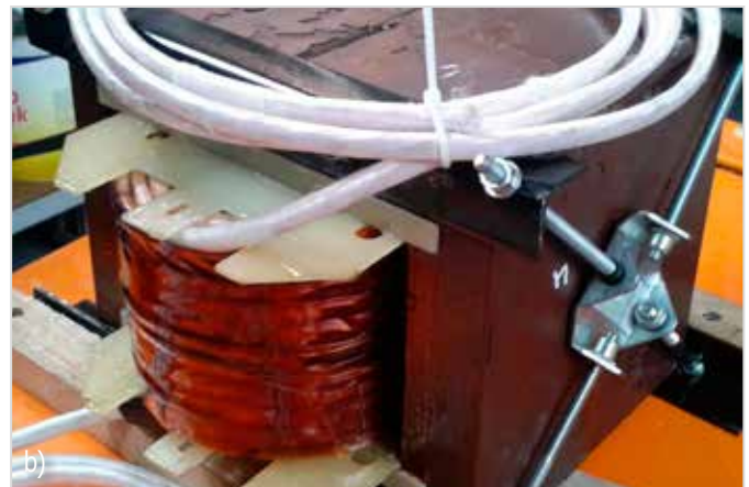
Figure 5. Examples of HF transformers made with Litz wire: a) 500 W rated with a ferrite core (Litz strands visible); b) 50 kW rated with a nanocrystalline core (Litz wire with 564 strands, 75 A)
