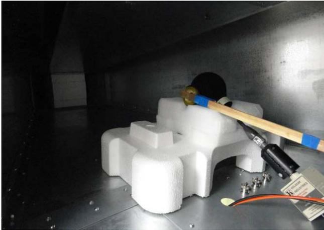
Fig. 14. Magnetic field probe calibration in GTEM TESEQ 750 cell using isotropic electric field probe HI-4455
