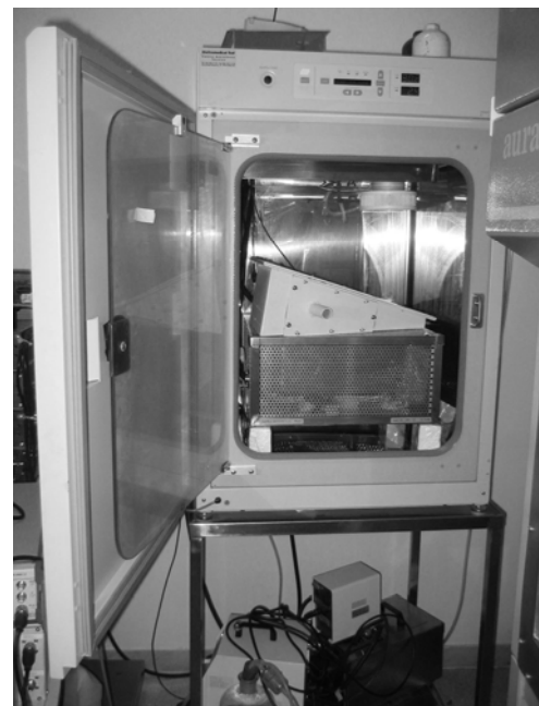
Fig. 5. Photo of the GTEM cell prototype located in the incubator.
