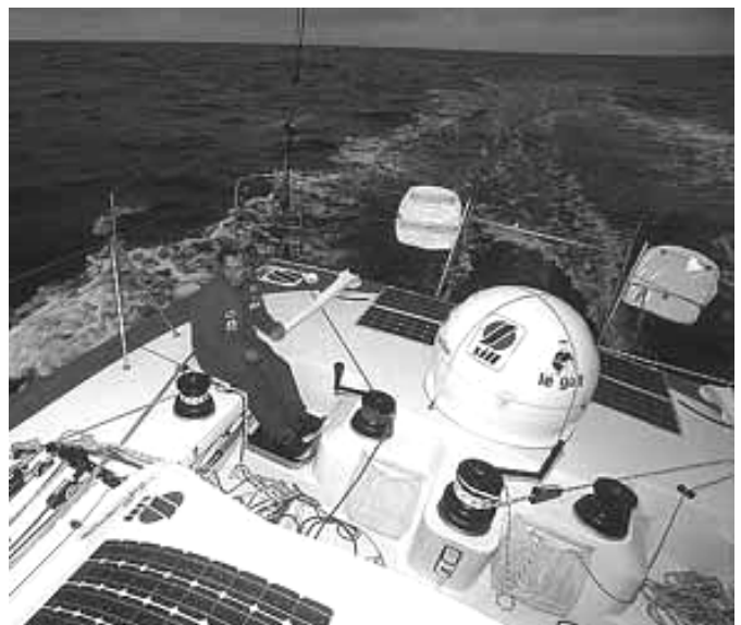
Fig. 5. Inmarsat antenna installed on the deck
