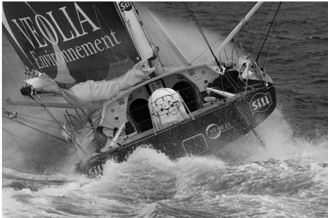
Fig. 6. Inmarsat antenna installed on the deck, ship rolling sideways by ca. 25^\circ
