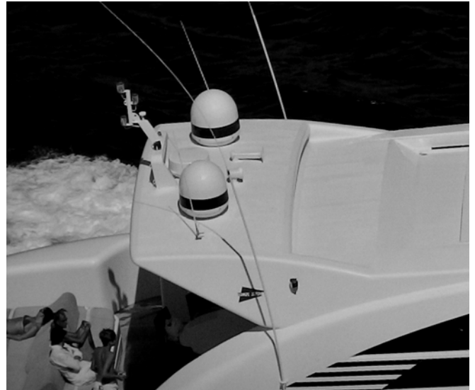
Fig. 4. Inmarsat antenna installed on the highest topside construction
