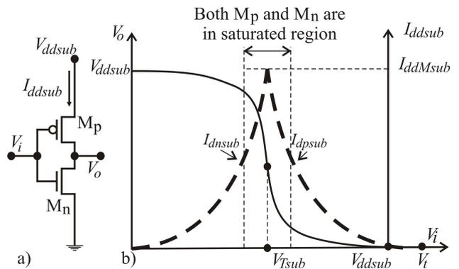
Fig. 2. CMOS inverter (a) and its  $V_o - V_i$  and  $I_{ddsub} - V_i$  static characteristics in sub-threshold region
