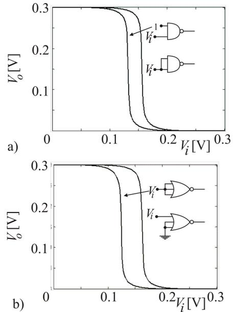
Fig. 4. NAND2 (a) and NOR3 (b)  $V_o - V_i$  static characteristics in sub-threshold operation region when only one input is active and when all inputs are active at  $V_{ddsub} = 300 \text{ mV}$
