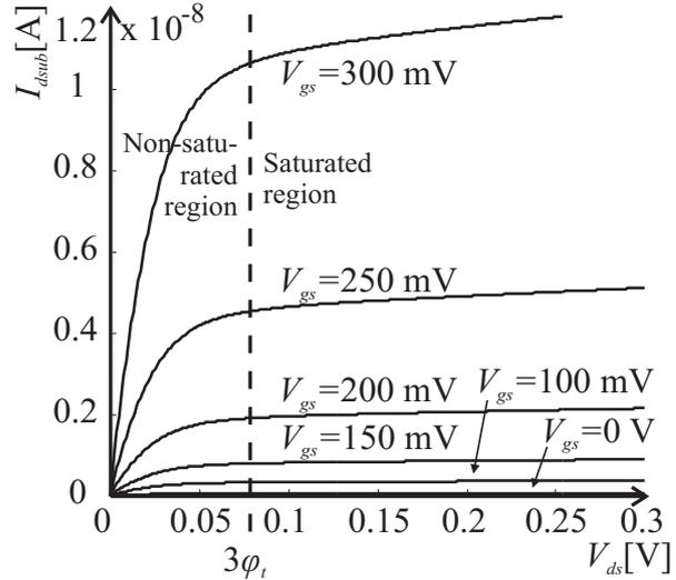
Fig. 1. MOS transistor  $I_{dsub} - V_{ds}$  characteristics in sub-threshold operation region [3]
