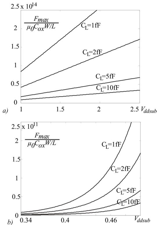
Fig. 7. Normalized  $F_{max}$  as a function of  $V_{dd}$ , shown for different values of  $C_L$ , when operating in strong (a) and weak (b) inversion region
