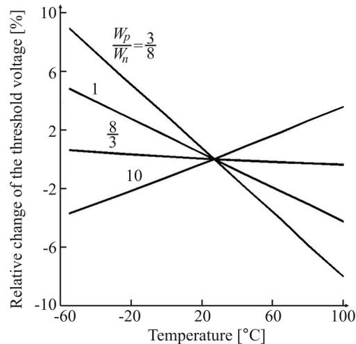
Fig. 8. CMOS inverter threshold relative change as a function of temperature for different ratios  $W_p/W_n$  (sub-threshold mode)
