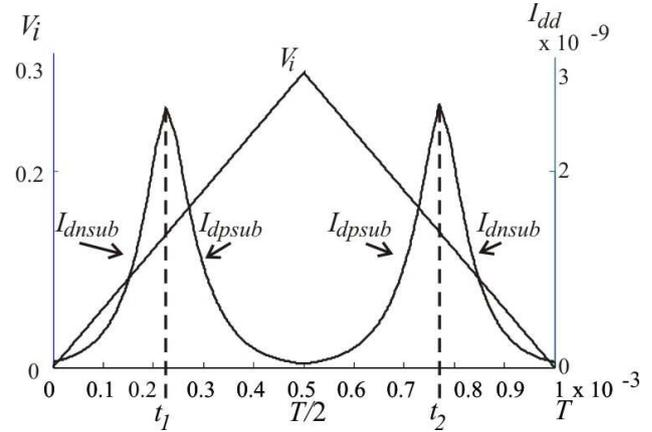
Fig. 11. CMOS inverter supply voltage current response to an input voltage linear change, when operating in sub-threshold [6]
