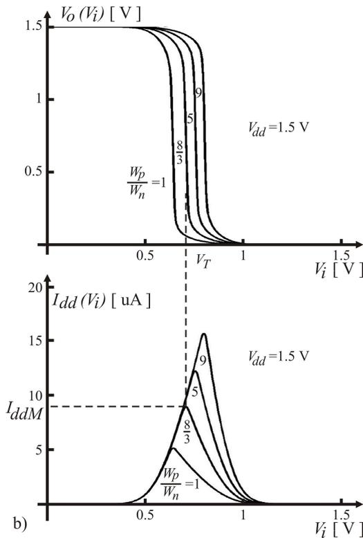
Fig. 3. CMOS inverter PSPICE voltage and circuit transfer characteristics in weak (a) and strong (b) inversion regime, where the ratio  $W_n/W_p$  is varied for the same  $L_n = L_p$
