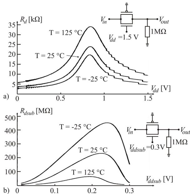
Fig. 12. The transmission gate resistance temperature dependence in standard operation mode at  $V_{dd} = 1.5$  V (a) and in sub-threshold at  $V_{ddsub} = 300$  mV (b) obtained by PSPICE analysis
