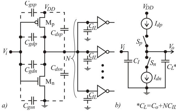
Fig. 5. CMOS inverter with corresponding capacitances (a) and its dynamic model (b) [6]
