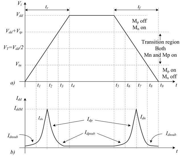
Fig. 10. The CMOS inverter transistor states (a) and the supply voltage current (b) at  $0 \leq V_i \leq V_{dd}$  (standard operation mode)
