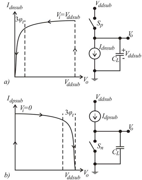
Fig. 6. Sub-threshold mode operating points trajectory and the equivalent circuits to charge (a) and discharge  $C_L$  (b)
