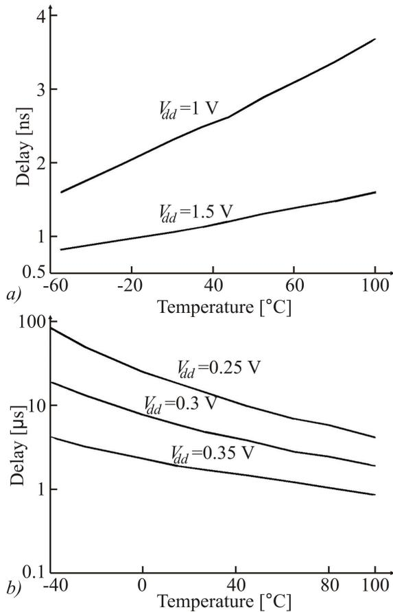
Fig. 9. The symmetric CMOS inverter delay as a function of temperature and supply voltage in: standard operation mode (a) and sub-threshold regime (shown in logarithmic scale) (b), at  $C_L = 20$  fF. The results are obtained by PSPICE circuit analysis
