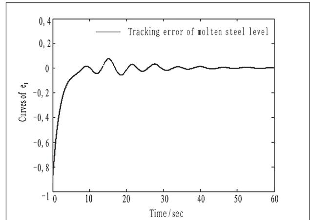
Figure 2 Trajectories of the state tracking error  $e_1$
