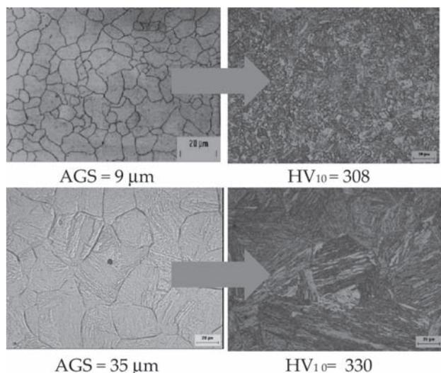
**Figure 4** Effect of AGS on microstructure after continuous cooling (steel S3,  $CR = 40\text{ }^{\circ}\text{C/s}$ ).
