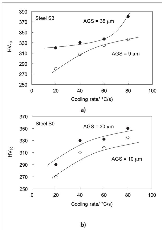
**Figure 6** Effect of AGS on hardenability a) Steel S0, b) Steel S3
