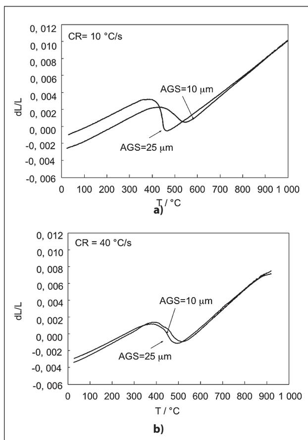
**Figure 5** Effect of AGS on length change of dilatometric specimens during continuous cooling: a) cooling rate =  $10\text{ }^{\circ}\text{C/s}$ ; b) cooling rate =  $40\text{ }^{\circ}\text{C/s}$  (steel S3).
