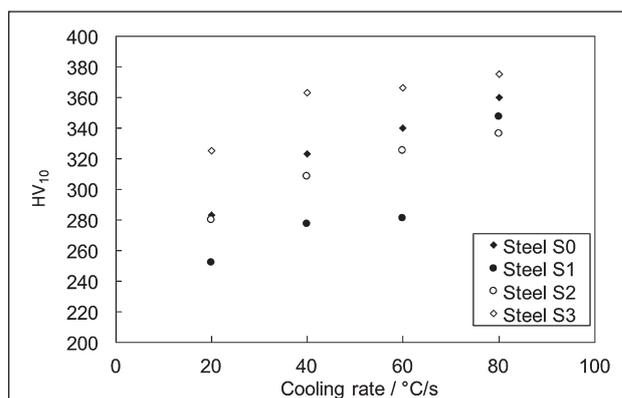
Figure 3 Hardness dependence on cooling rate.
