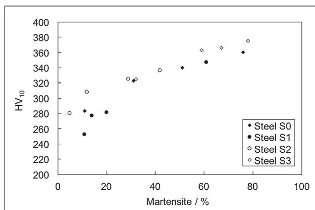
Figure 2 Hardness dependence on martensite volume fraction
