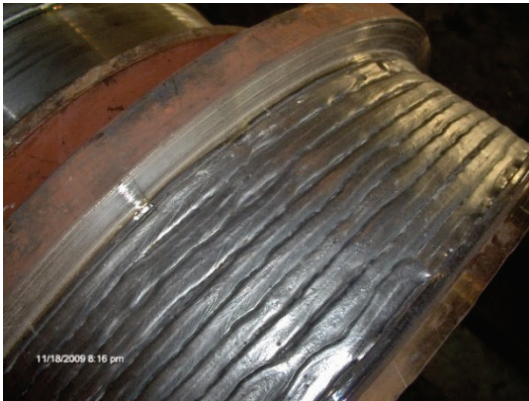
Figure 7 Repaired wheel after welding procedure
