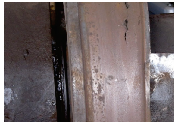
Figure 6 Rim wear and breakage during the wheel exploitation
