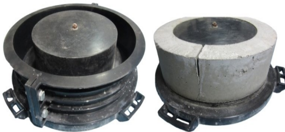
Figure 1. Novel restrained shrinkage ring mould and cracked sample.
