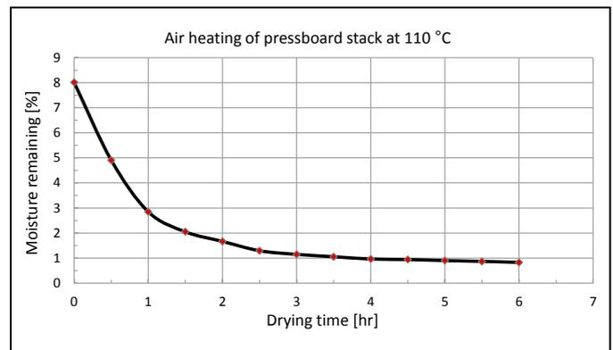
Figure 3. Moisture remaining in the pressboard stack (consolidated) over time
