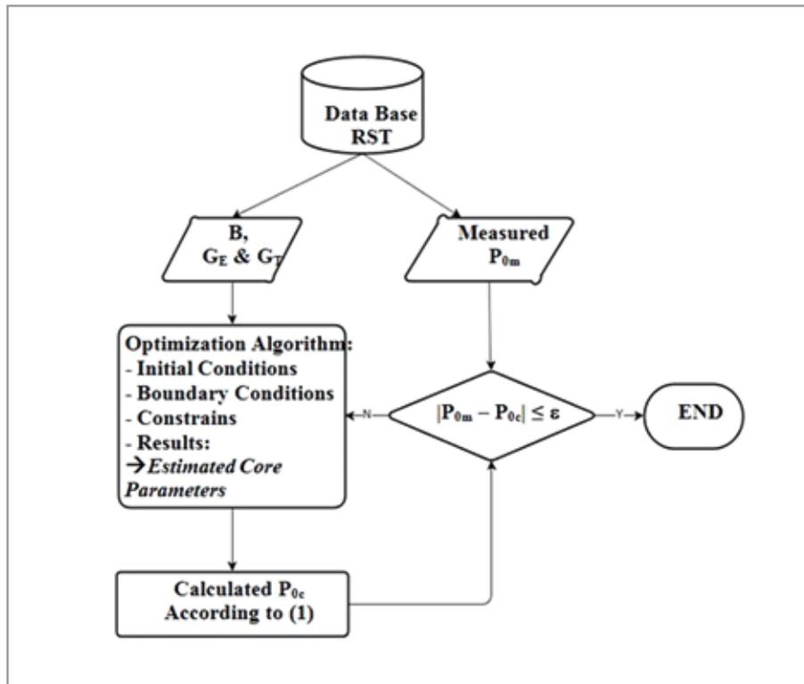
Figure 4. Flow chart for determining core parameters of Reference Sheet Type
