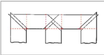
Figure 3. 45° mitre overlapped construction
