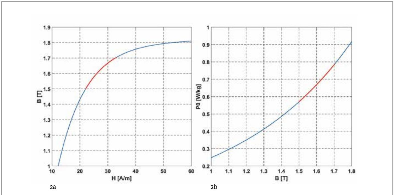
Figure 2. (a) Example of hysteresis curve ( $B$ - $H$  curve); (b) The corresponding specific no-load loss curve against flux density (red coloured region for flux density between 1.5 and 1.7 T)
