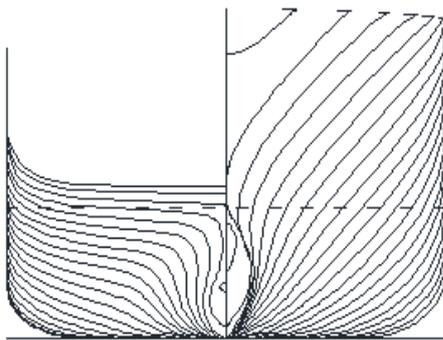
**Fig. 3** Lines plan for the C11 containership
