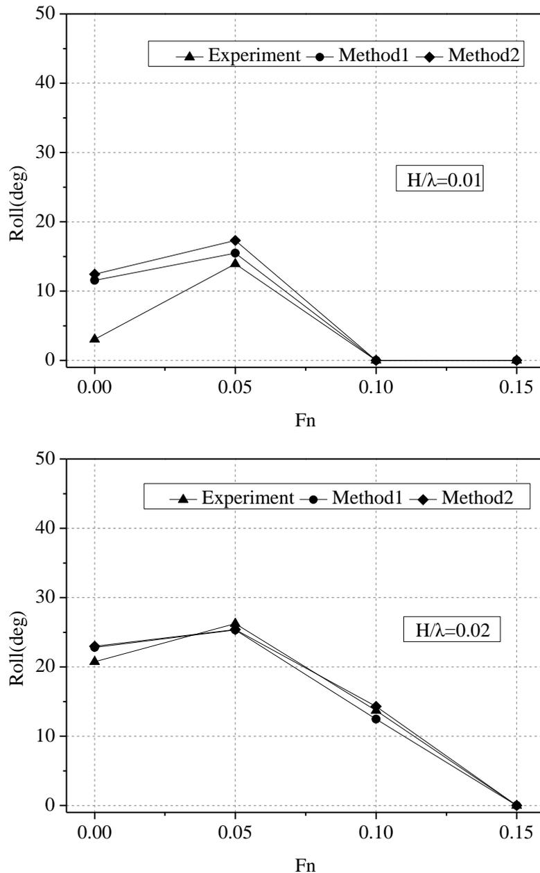
**Fig. 12** Comparison of steady roll amplitudes between experimental measurements and numerical simulations using different roll damping prediction methods for the incident wave steepness  $H/\lambda = 0.01, 0.02$ .
