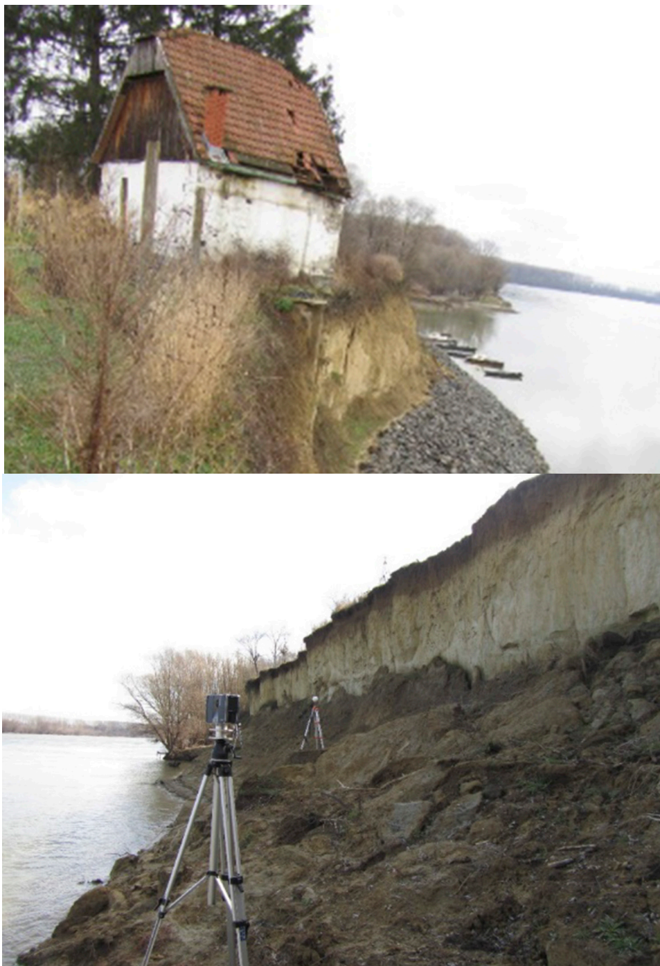
Figure 5. Vacation home endangered by erosion (left) and laser scanning of the bank (right).
