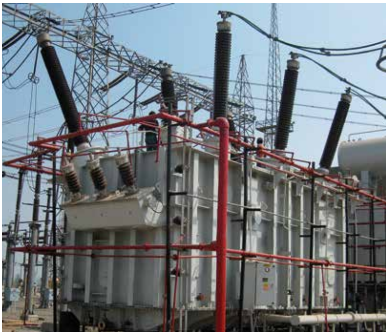
Figure 9. The unit under test and its representation in the localisation software, with sensors visible at the top and the three tap changer compartments highlighted in brown
