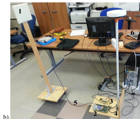
Fig. 2. a) Architecture of the proposed RFID tag characterization system. b) Measurement setup: 1. Reader antenna, 2. Reader board 3. Driver Board, 4. Stepper Motor, 5. Coax Cable.
