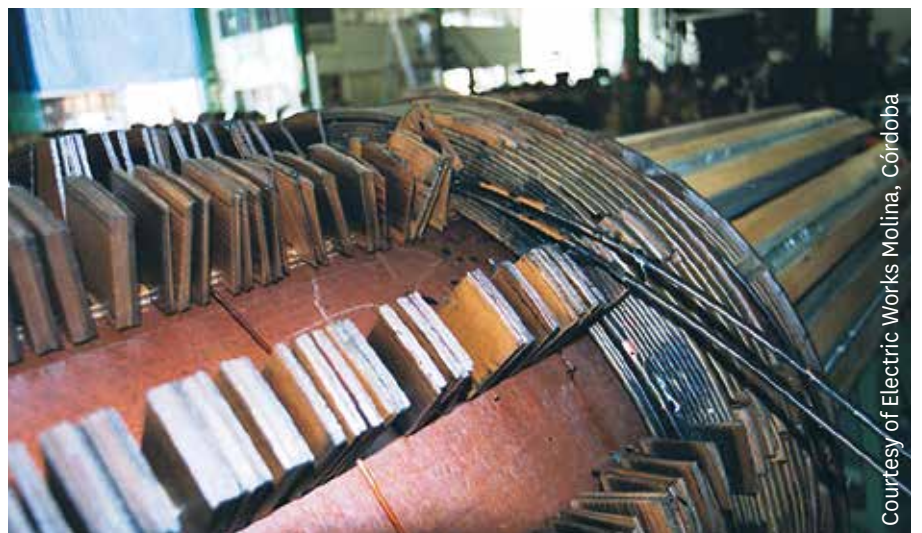
Figure 1. Breakdown of the dielectric system in a power transformer column
