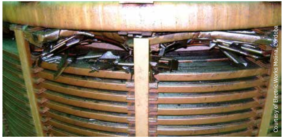
Figure 10. Collapsed winding degradation detectable with FRA
