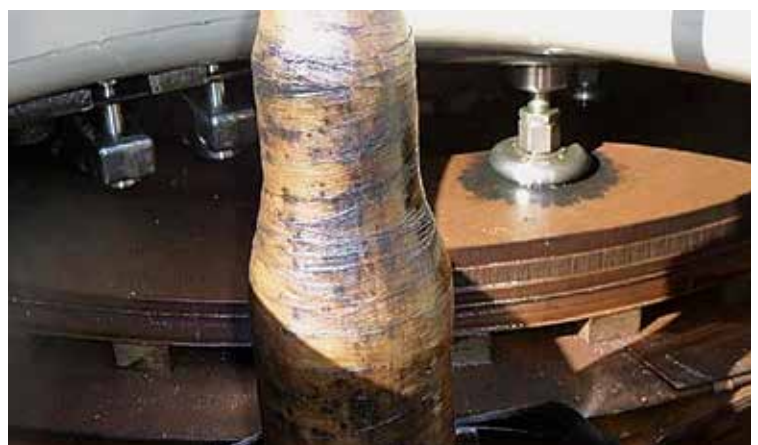
Figure 11. Traces of PD at the bushing lead
