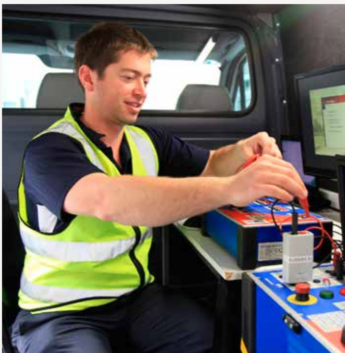
Site acceptance testing is a critical requirement for ensuring the transformer’s condition and preparedness for service.
