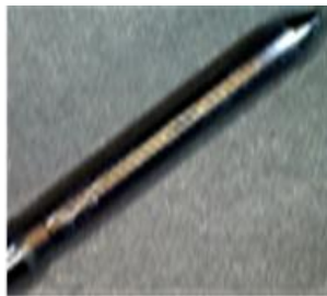
Figure 7: Amide Injector Deposit. Polymeric based, brown in colour
