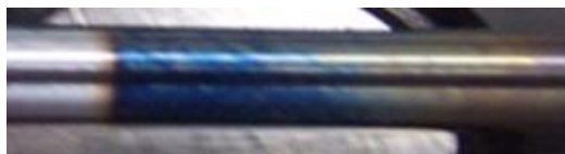
Figure 9: Lacquer Based. Visualised on some injectors, may be a carbonaceous deposit precursor
