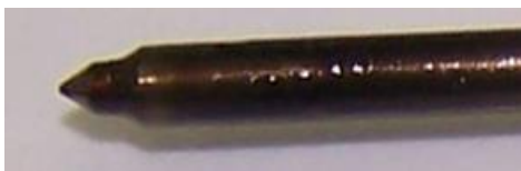
Figure 8: Aged Fuel Deposit, 'sticky' deposit possible bio in origin
