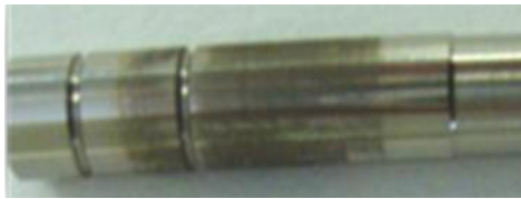
Figure 6: Carbonaceous Injector Deposit. Carbon Based, black in colour
