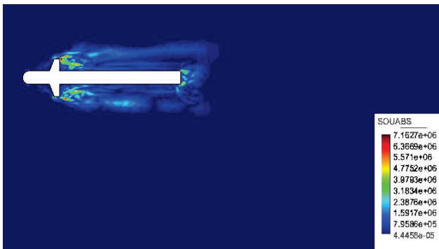
Figure 15 Absolute source field around missile, using LES approach in the XZ plane
