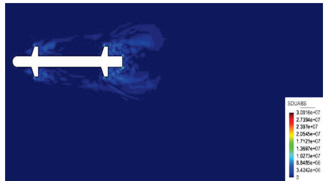
Figure 19 Absolute solution of source field around missile using LES approach in the XY plane
