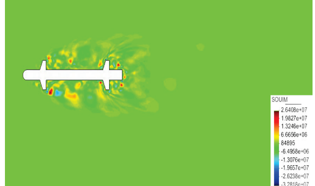
Figure 22 Imaginary solution of source field around missile using DynOSS approach in the XY plane
