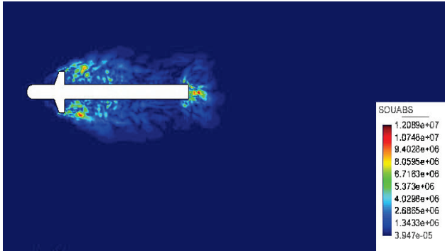
Figure 16 Absolute source field around missile, using DynOSS approach in the XZ plane
