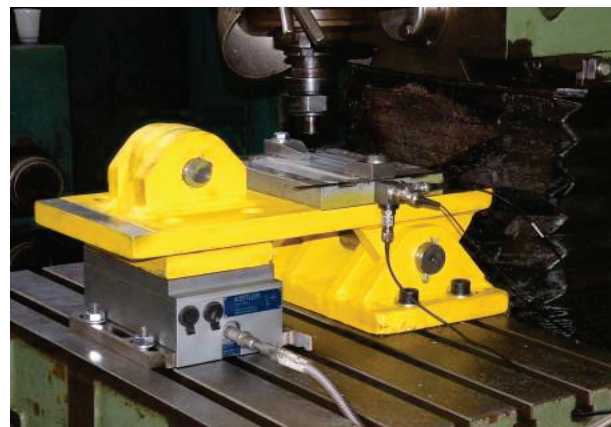
Figure 5 Experimental welding with welding power and tool oscillations measurement system
