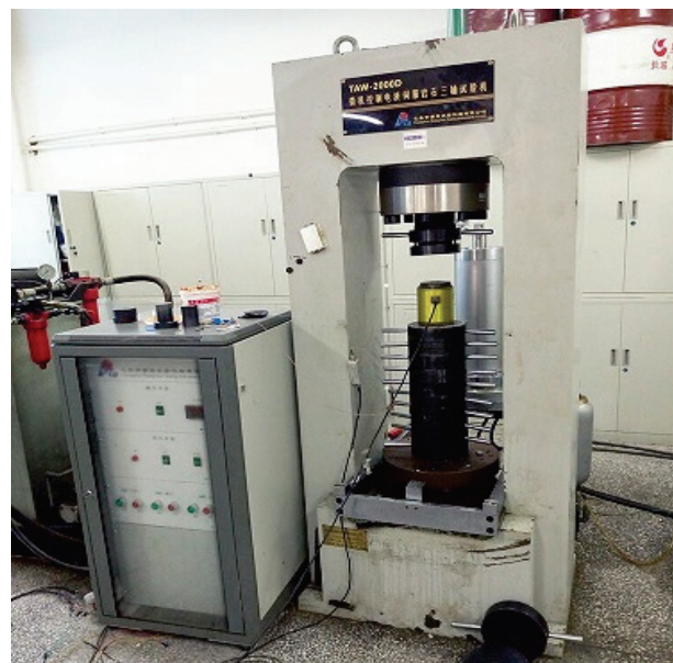
Figure 2 TAW-2000D microcomputer-controlled electro-hydraulic servo rock triaxial compression testing machine
