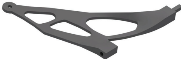
Figure 17 Optimal shape of L-shape MacPherson control arm
