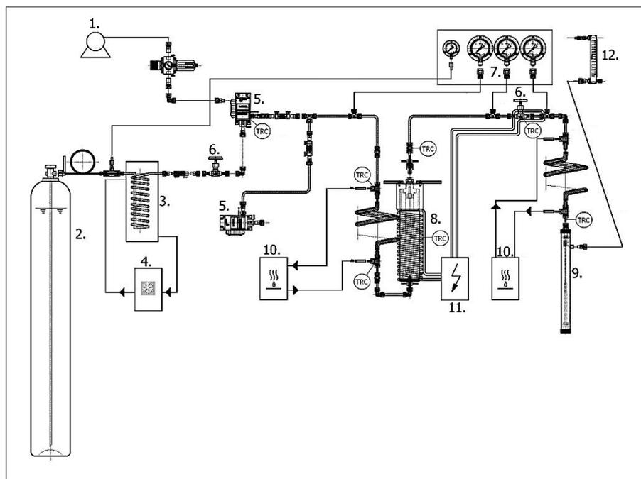
**Figure 1** Handmade supercritical fluid extraction system
