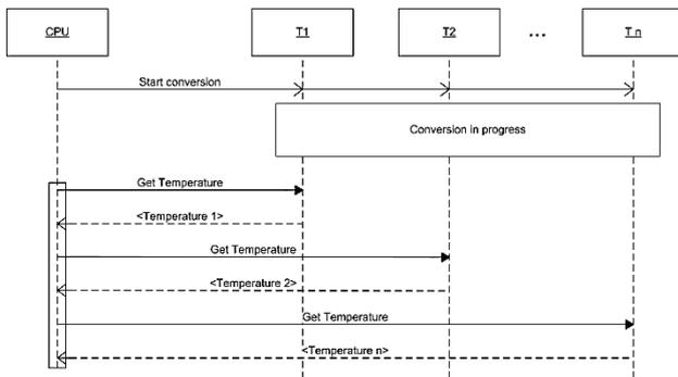
Figure 4 Sequence diagram of the temperature sensors data acquisition
