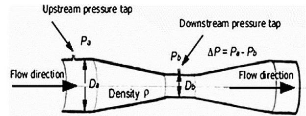
Figure 3 Cross-section of a venturi nozzle [13]
