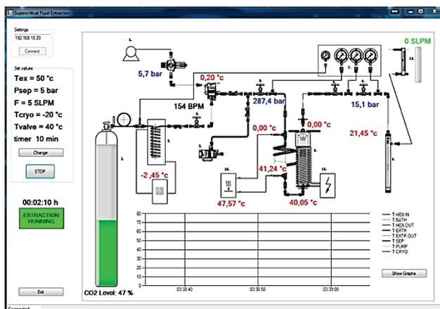
Figure 13 Developed PC application for the HM-SFE system
