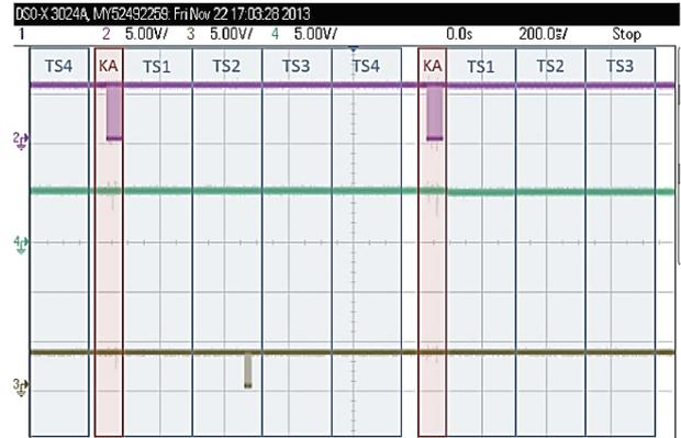
Figure 9 Application (Slave 2) transmits a write request (2 - data transmit from Master, 3- data receive on Master, 4 - data transmit from user interface)
