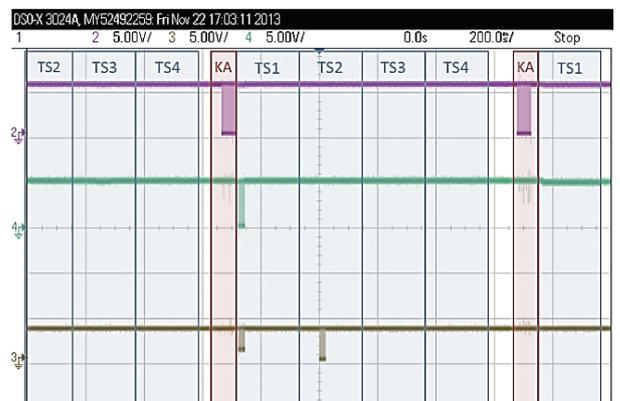
Figure 11 Both application (Slave 2) and user interface system (Slave 1) transmits a write request (2 - data transmit from Master, 3 - data receive on Master, 4 - data transmit from user interface)
