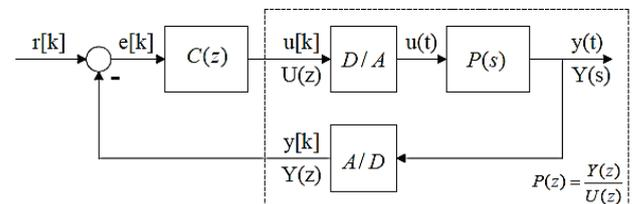
Figure 5 Controlling continues process by discrete regulator
