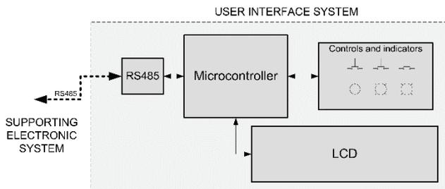
Figure 12 User interface system for SFE device
