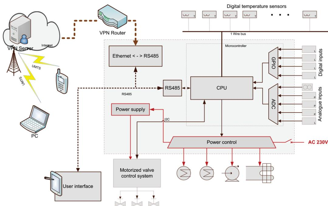
Figure 2 Block diagram of the supporting electronic system
