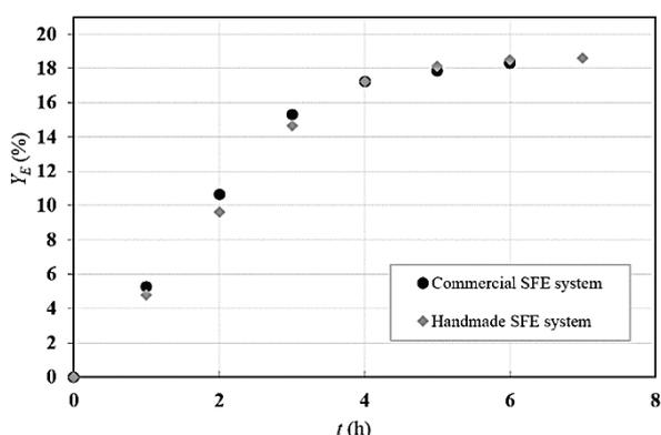
**Figure 14** Extraction yield of soybean oil obtained by supercritical CO<sub>2</sub> at the commercial and HM-SFE system. Conditions:  $T_E = 40$  °C;  $P_E = 40$  MPa;  $m_f = 0,476$  kg/h
