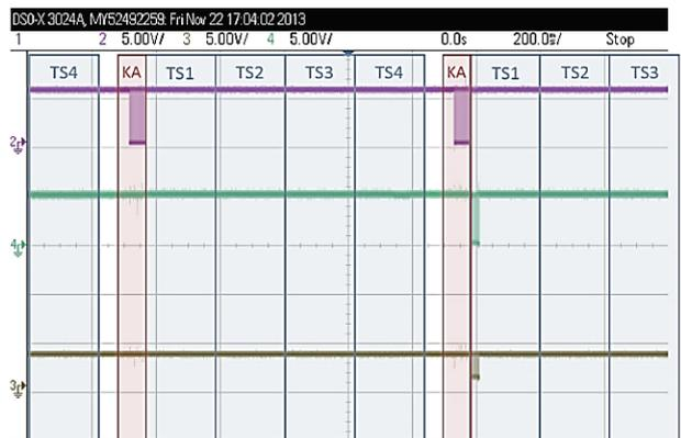
Figure 10 User interface system (Slave 1) transmits a write request (2 - data transmit from Master, 3- data receive on Master, 4 - data transmit from user interface)
