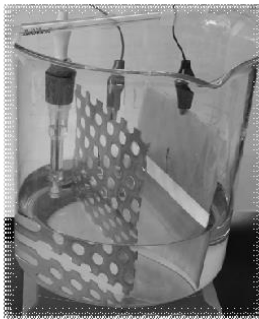
Figure 1. Glass cell containing Ti mesh counter and SCE reference electrodes used for determination of electroactive area of working electrodes (Al, Fe, G, Ti/RuO 2 )
