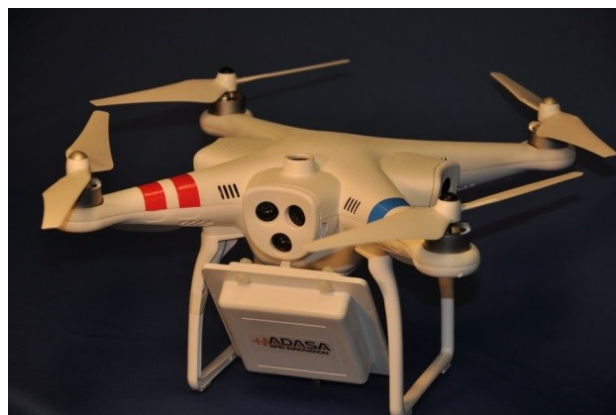
Figure 10. A flying robot by the company ADASA capable of RFID scanning [29].
