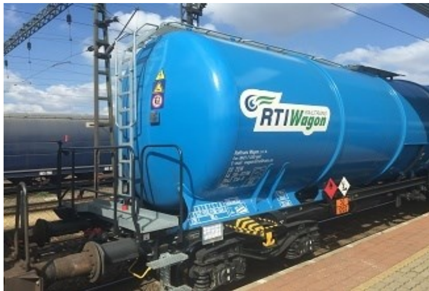
Figure 2. Visual marks on a tank wagon referring to the transported goods.
