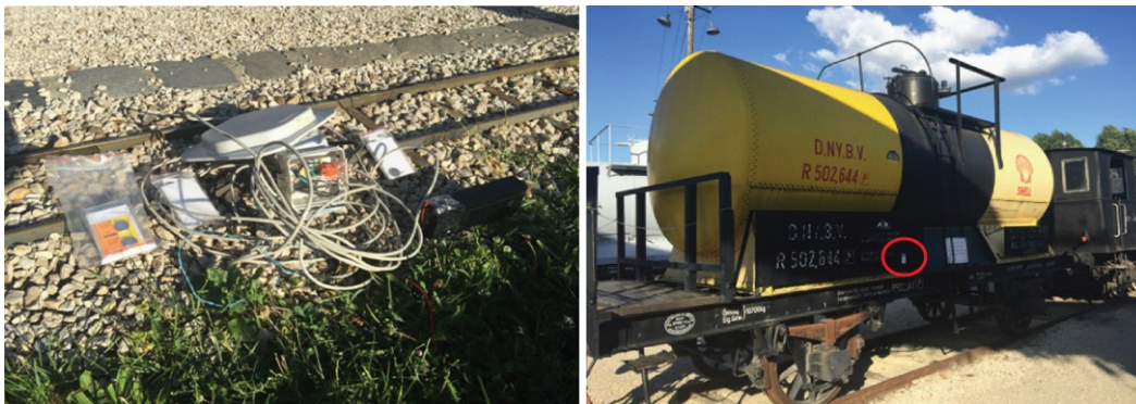
Figure 13. Devices of the experiment and the tank wagon with its tag (in red circle).
