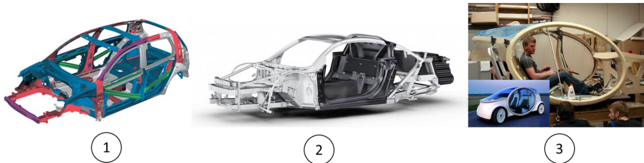
Figure 6 Comparison of automotive body types with different materials. 1: standard steel body (Volkswagen Golf [9]), 2: aluminum space frame technology with carbon fiber components (Audi R8 e-tron [10]), 3: prototype of a wood frame vehicle body (Nios [11])
