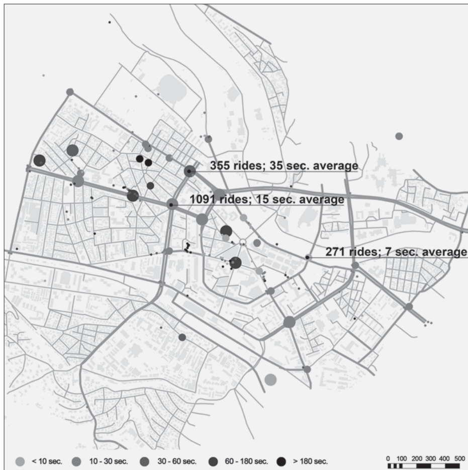
FIG. 5 THE SPOTS WITH CONGESTIONS AND DOWNTIMES DURATION. THE RESULTS ARE SHOWN AS SPATIAL RELATION OF SPOTS CLASSIFIED ACCORDING TO THE DURATION OF CONGESTION IN THE SECTION OF THE TRAFFIC NETWORK (CONGESTION WITHIN THE PRIMARY, SECONDARY OR THE CROSSING OF THE TWO TRAFFIC NETWORKS). USING A SET OF DATA REPRESENTED ON COMMUTE ROUTES LAYER OVER A GRID SUBSTRATE THE NUMBER OF STOPS AND THE AVERAGE DOWNTIME IN ANY OF THE FIELDS WERE CALCULATED. ALL POINTS WITH A MINIMUM OF 10 DELAYS WERE TAKEN INTO CONSIDERATION, IN ORDER TO AVOID THE INDIVIDUAL OR UNUSUAL. THE RESULT INDICATES THE TOTAL NUMBER OF STOPS IN EACH OF THE GRID FIELDS. DOTS THAT SHOW THE AVERAGE TIME OF STOPPING ARE INDICATED WITH DIFFERENT SHADES, WHILE THE NUMBER OF INDIVIDUAL STOPS IS REPRESENTED BY VARIATIONS IN THE SIZE OF THE CIRCLE/DOTS. THE MAP REPRESENTS THE TOTAL NUMBER OF STOPS IN TERMS OF DURATION OF CONGESTION. THREE POINTS WITH EXACT NUMBER OF STOPS AND AVERAGE TIME SPAN OF SLOWDOWN ARE PRESENTED ON THE MAP.
