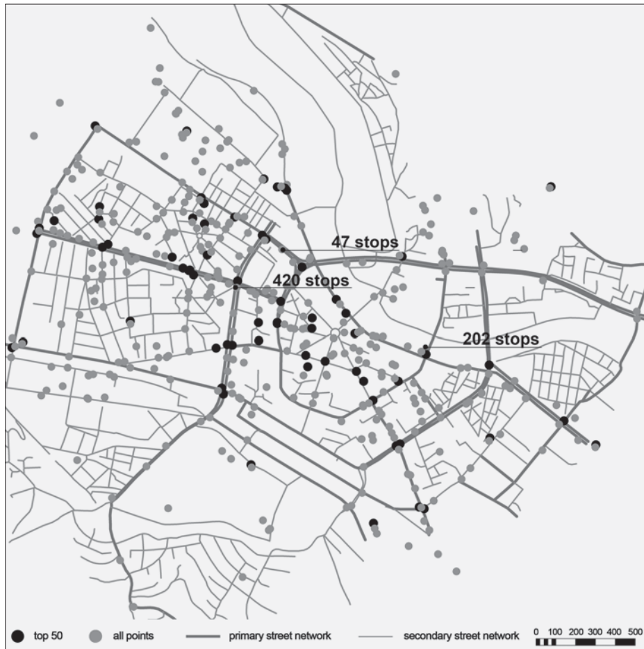
FIG. 4 DENSITY OF POINTS OF DOWNTIME, COMMUTE ROUTES LAYER. DESCRIBED ARE THE DENSITY AND PLACES WHERE OBSTACLES SLOWED DRIVES BUT DID NOT STOP THEM, WHILE ANALYSING A RANGE OF ASPECTS SUCH AS DURATION, REPETITION IN VARIOUS DRIVERS AND RANK OF THE STREET NETWORK. SINCE THERE ARE MORE THAN 400 POINTS, ONLY 50 POINTS WITH BIGGEST FREQUENCY OF SLOWDOWN ARE PRESENTED FOR THE PURPOSE OF BETTER VISUALIZATION, WHILE THREE POINTS WITH EXACT NUMBER OF STOPS/DOWNTIME ARE PRESENTED ON THE MAP.
