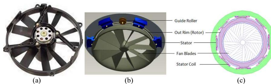
Figure 1. Structure of fan motors: (a) Traditional; (b) Prototype and (c) cross section of new distributed
