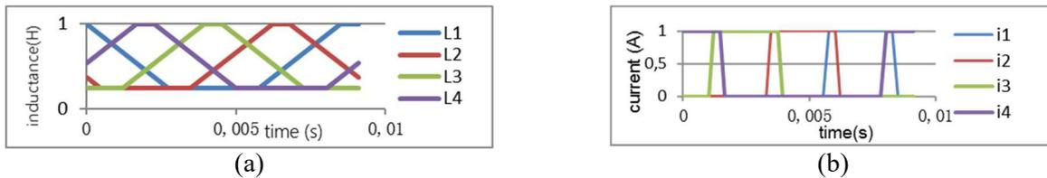
Figure 6. Ideal profile for (a) inductance; (b) current of designed SRM
