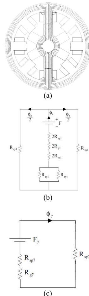
Figure 9. (a) Flux paths; (b) equivalent circuit for mutual path 1; (c) equivalent circuit for path 7 at aligned position [16]
