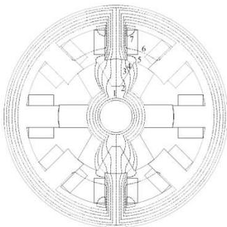
Figure 10. Flux paths for unaligned position [16]
