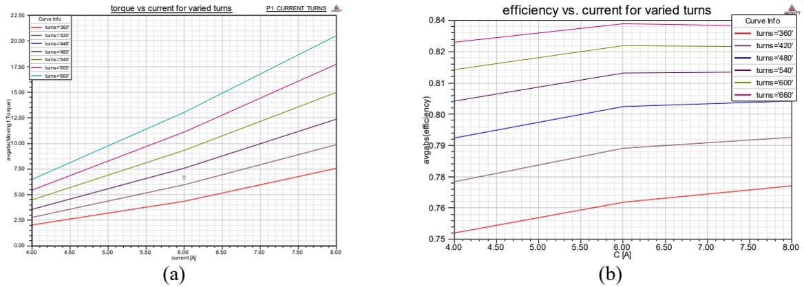
Figure 7. FEA results for (a) torque (b) efficiency vs. phase current for varied winding turns per phase
