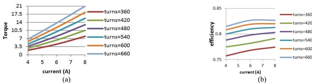
Figure 4. Relationship curves between (a) torque and (b) efficiency vs. excitation current for various turns per phase.
