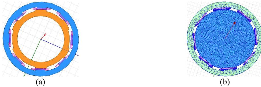
Figure 5. FEA models for (a) geometry (b) mesh
