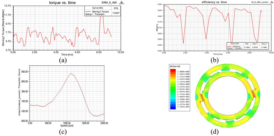
Figure 8. Characteristic features of a design: (a) torque vs. time; (b) efficiency vs. time; (c) output power vs. speeds; (d) flux density distribution at aligned position.
