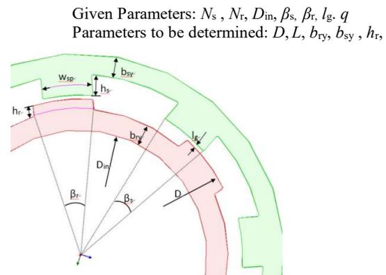
Figure 2. Parameters for SRM design
