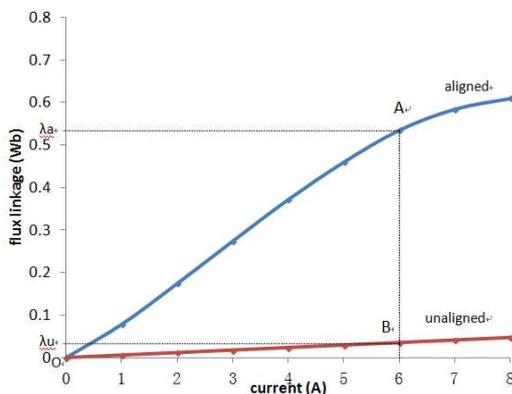
Figure 3. Magnetization curve for the initial designed SRM
