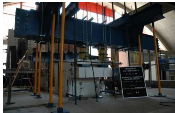
Fig. 2 System of load application
