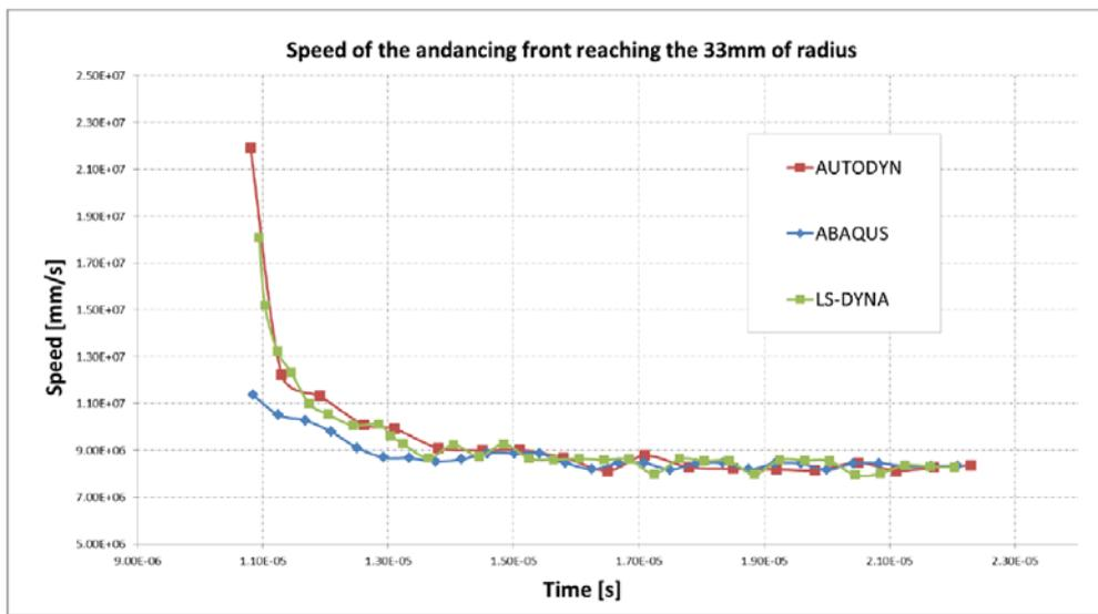
Fig. 8 Advancing speed of the front
