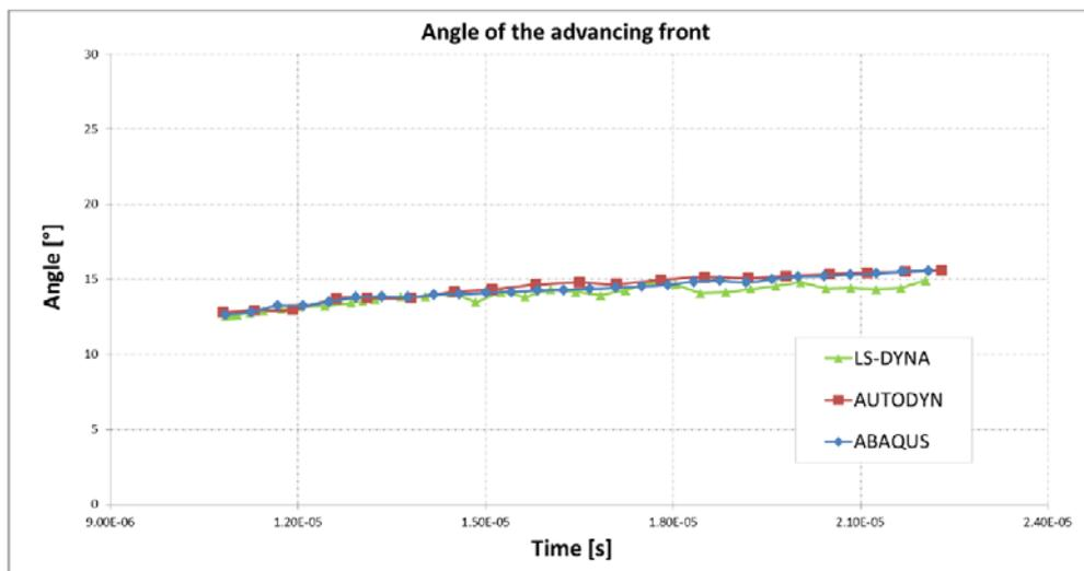
Fig. 9 Angle of the deformed tube wall
