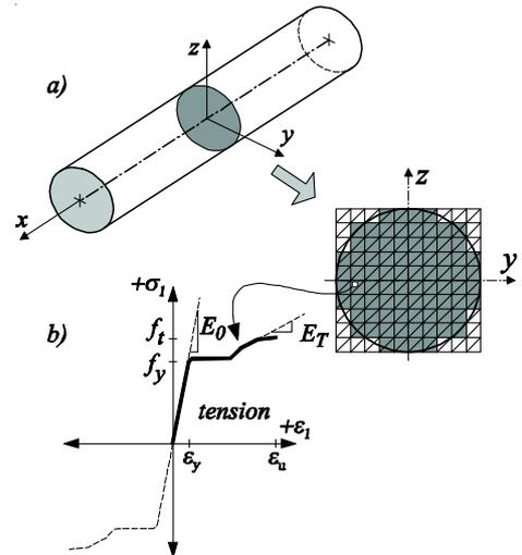
Figure 3 Modeling of cross-section:
