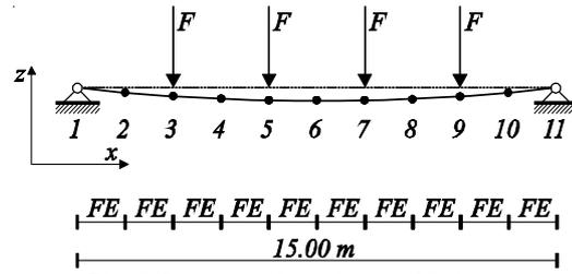
Fig. 6 Structure discretized by 10 elements
