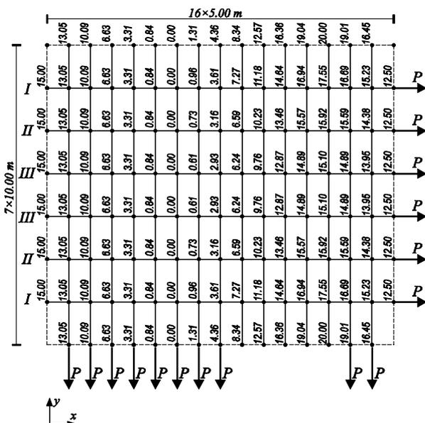
Fig. 14 Saddle net: startup geometry and first phase loading
