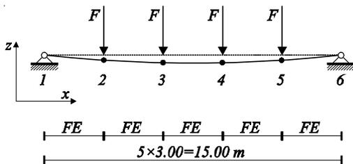
Fig. 5 Structure discretized by 5 elements
