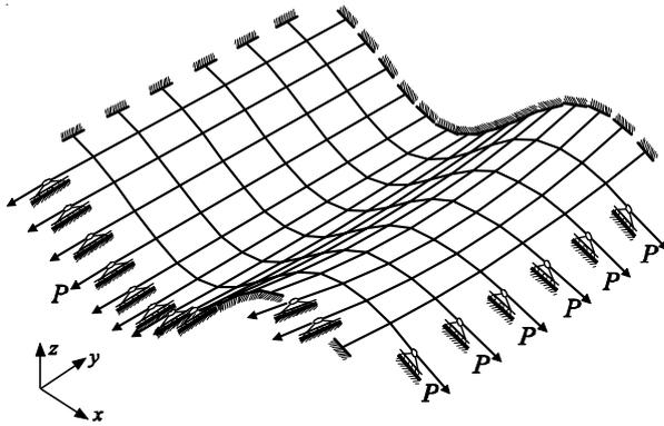
Fig. 13 Saddle net - isometric view with first phase loading
