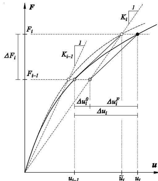
Fig. 1 Symbolic description of large displacements of single degree-of-freedom system
