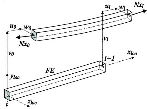
Fig. 2 Tensile two-noded space finite element
