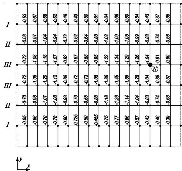
Fig. 15 Saddle net: values of displacement in global z direction (m) for the ultimate load
