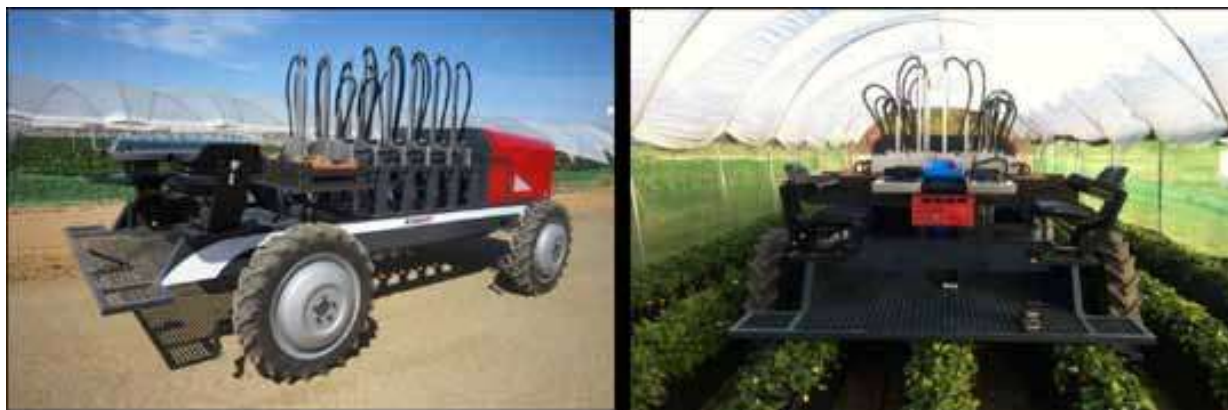
Fig. 7. AGROBOT SW 6010 harvester or robotic strawberry picker
