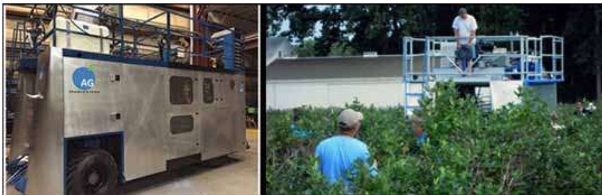
Fig. 1. AGH 3000 top loading mechanical harvester being used on blueberry fields
